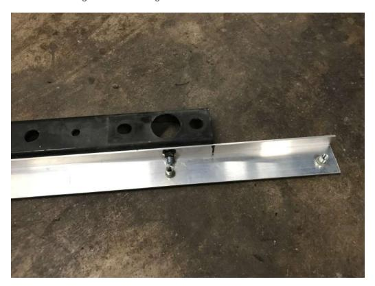
Attach Differential Bracket as shown. Angle so that bottom edge is parallel to ground. Keep diff side bolt slightly loose to make adjustments.
