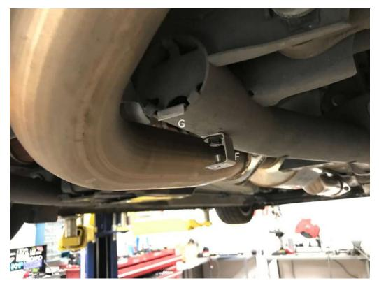
Remove Rear center clips from bumper. Attach C brackets in place of clips as shown. (lower edge outward and parallel to ground.) Leave upper portion loose.
