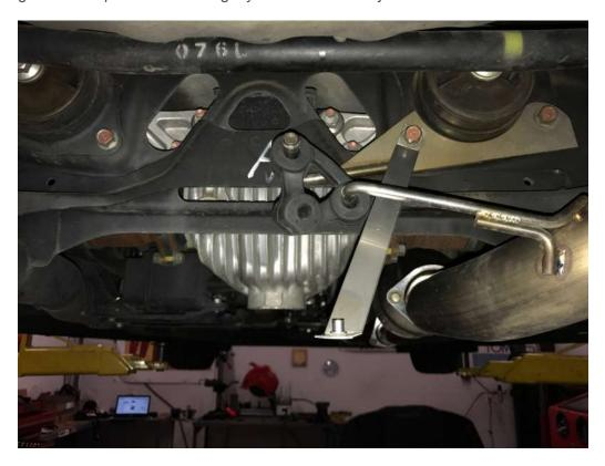
Attach 2BL (rear) and 2AL (front) brackets along driver edge of bumper as shown. Keep upper edge loose until end.
