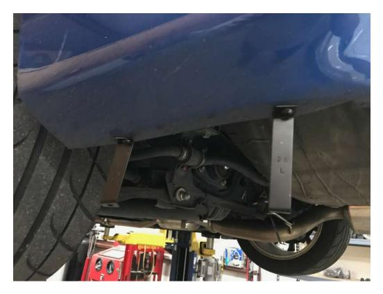
Slide G Bracket into subframe, attach F Bracket (facing open end towards center of car).
